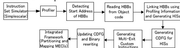
Fig. 6. Tool chain for generating MECIs
