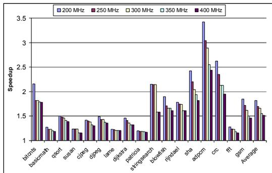
Fig. 12. Effect of the clock frequency on speedup
