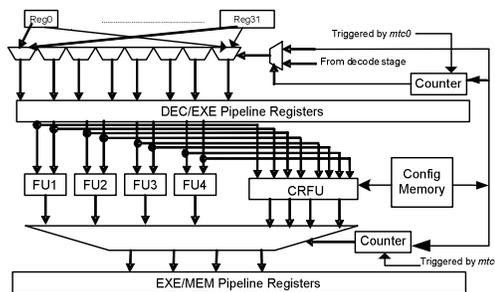
Fig. 1. Integrating the base processor with the CRFU
