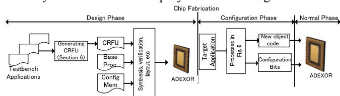
Fig. 2. Different phases for designing and using ADEXOR
