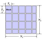
Figure 3. Dividing a two-dimensional array into data blocks (tiles). All the data blocks have the same size except possibly at the boundaries of the array.
