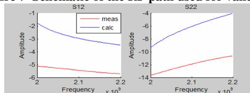
**Figure 8 Comparison of calculated and measured S-parameters**
