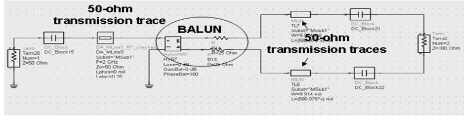
Figure 4 RF-path on load board
