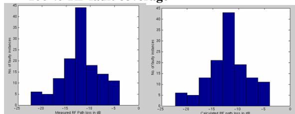
**Figure 6 Distribution of measured and calculated path loss for multiple faulty instances**
