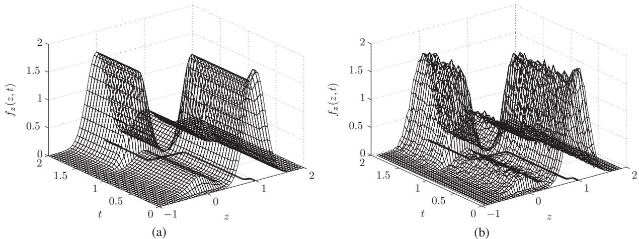
Figure 3. Pdf of output signal derived (a) analytically and (b) simulated.
