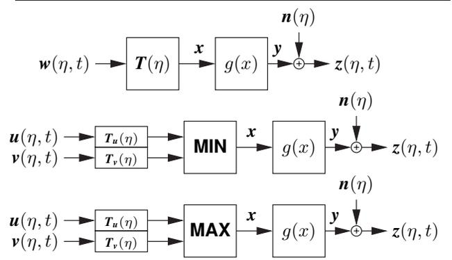
**Figure 2. Composition of logic gates from presented BBBs. From top down: NOT-, NAND- and NOR-gate.**
