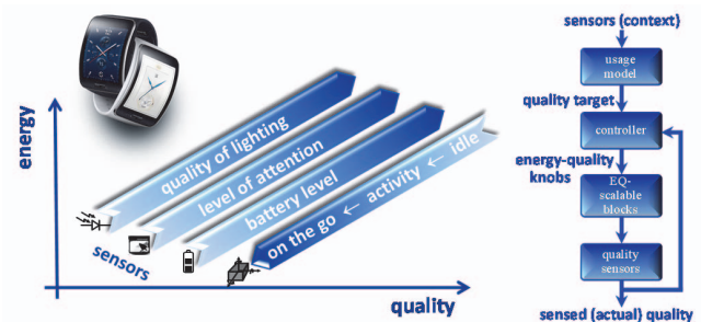
Fig. 5. Opportunities to scale down quality and energy in a smartwatch delivering video content, under poor quality of lighting, low level of user's attention, low battery level, high level of physical activity.
