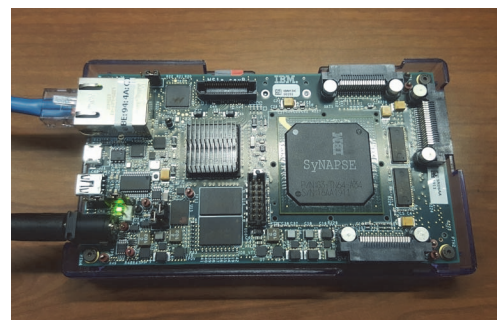
Figure 1. NS1e development platform with a single IBM TrueNorth processor.
