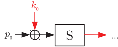
Fig. 3. UPTA-like plaintext recovery attack on one plaintext byte in the first AES round. Two templates, one on the whitening key k_0 and one on the S-box output S(p_0 \oplus k_0) , have to be trained.
