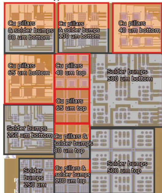
Fig. 2: Test vehicle layout developed on purpose (top and bottom dice)
