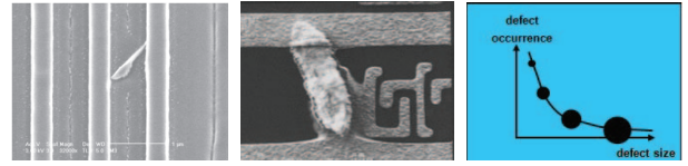
Fig. 1. Examples of disturbing bridges. Connections with small resistors values can lead to large defects to the solution.
