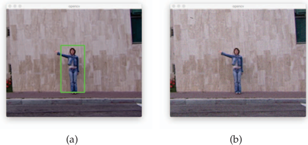
Fig. 1. (a) A human detection algorithm based on the histogram of oriented gradients (HOG) implemented using the OpenCV library correctly reports that the video frame on the left has a human. (b) The same OpenCV implementation of the human detection algorithm reports that the video frame on the right has no human. The video frame on the right is obtained by adding tiny perturbations to the left video frame. Both frames look identical to the naked eye.
