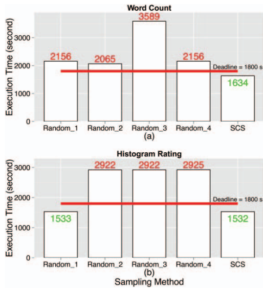
Fig. 7. Impact of estimation accuracy on deadline and resource usage
