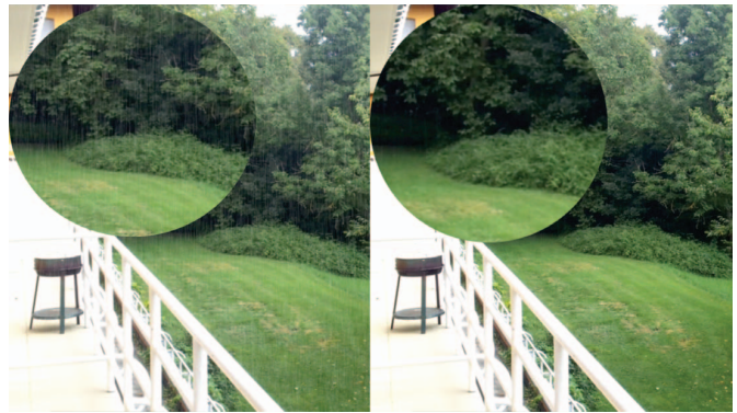
Fig. 2. Rain with an artificial depth map. The depth map contains two levels of depth for illustrative purposes, containing higher depth values in the left part. The number of drops between a scene object and the virtual camera depends on the scene depth. Therefore, in the left part, more drops are visible than in the right part.
