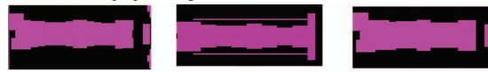
Fig. 12: Portion of B2 OPCed Mask outputted from: (a) Algorithm proposed in [4]. (b) PVOPC [15] (c) Our proposed algorithm.
