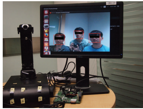
Fig. 4. Telepresence robot running real-time face detection on Jetson TK1
