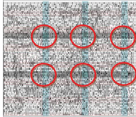
Fig 5. Floorplan of standard PDN with via insertion (in red)
