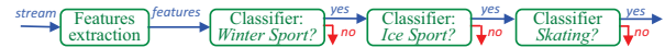
Fig. 1. Example of stream mining application for ice-skating detection [3] the workload by selecting the percentage of data that will be processed while other approaches [1][2][3][4] control the processing method of the data streams to adapt to the given allocated resources. However, these approaches had very limited considerations to the dynamic characteristics of the data streams, which may experience concept drift [11] and thus require continuous adaptation. Approaches that rely on offline information are not able to adapt to these concept drifts online.
