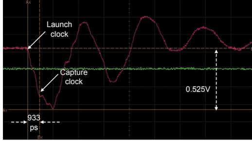
Figure 1. VDD power droop observed on ATE.
