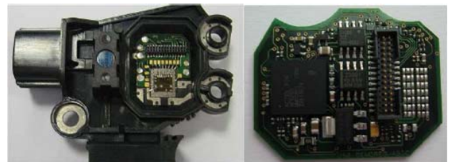
Figure 6. Assembled brush holder with the IC (left) and mezzanine board with the FPGA (right)
