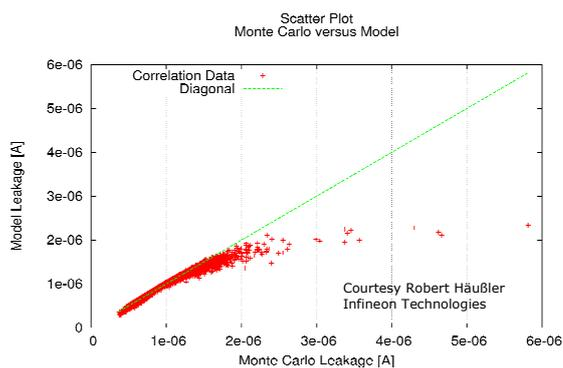
Figure 3. Comparison Monte Carlo simulation vs. log-linear leakage model for a 90nm inverter at 135°C
