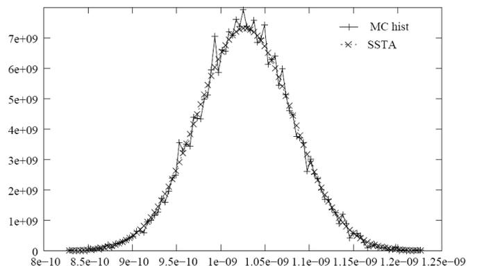
Figure 2. Comparison of Monte Carlo histogram and Gaussian probability density function obtained by the proposed method
