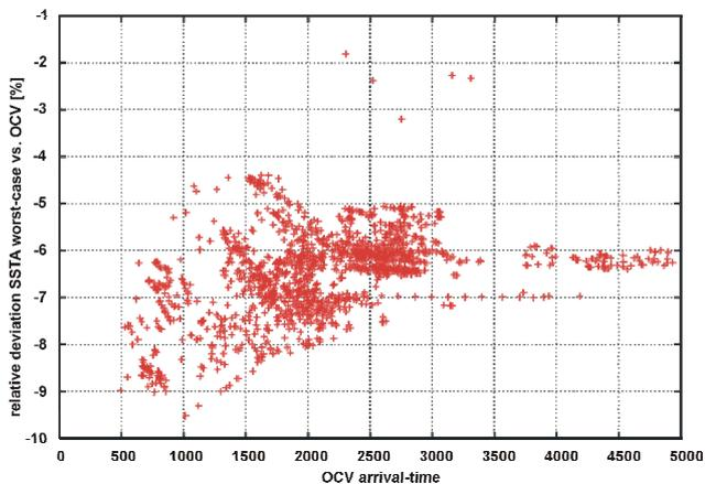
Figure 1. Relative deviation (in %) of timing-path arrival times reported by STA + OCV compared to highly accurate SSTA.
