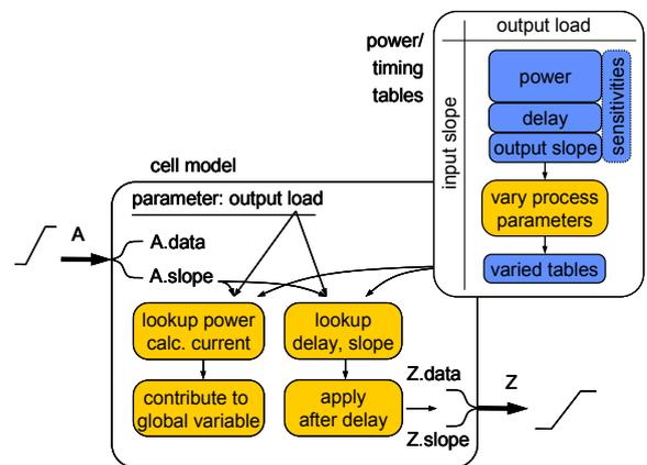
Figure 4. VHDL Cell model structure for statistical power simulation
