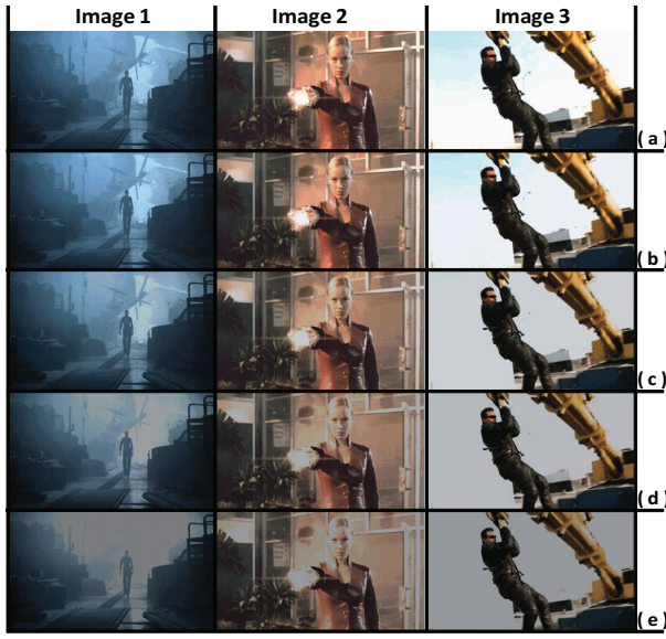
Fig. 7. Images at different distortion levels: a) Original images; b) High quality (SSIM = 0.98); c) Medium quality (SSIM = 0.96); d) Low quality (SSIM = 0.94); e) Unacceptable (SSIM = 0.90).
