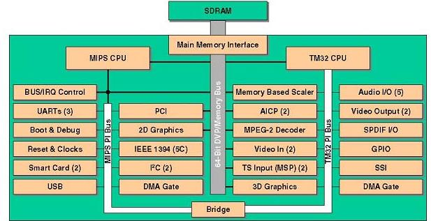
Figure 4. Block diagram of one NXP DTV SoC
