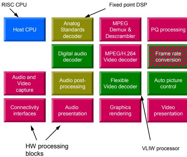
Figure 1. Application mapping
