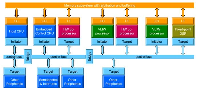
Figure 3. Conceptual view multi-core SoC architecture
