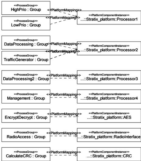
Figure 4. Mapping process groups to processing elements.
