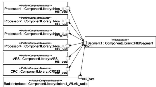
Figure 3. Architecture model of a platform instance.
