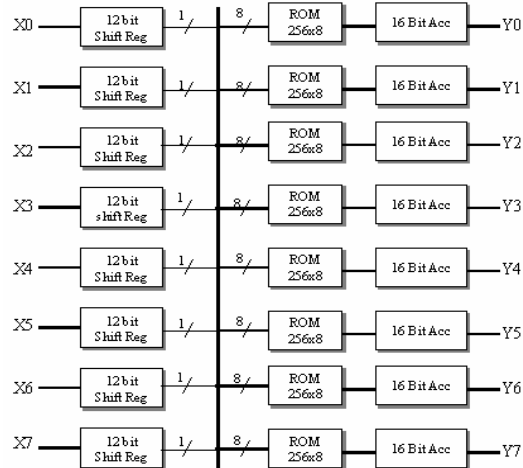
Figure 9: Implementation of Li's Algorithms with larger LUTs but not adders and subtractors at the input.
