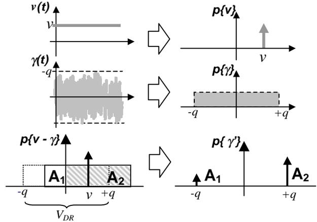
**Figure 2: Acquisition with dithering. Signal ( $v$  – a constant value) and noise ( $-\gamma$ ) PDF's are convoluted and area sampled by the 1-bit AD. Statistics before and after quantization are related, and the resulting bit-stream ( $\gamma'$ ) can be used to infer properties  $v$ .**
