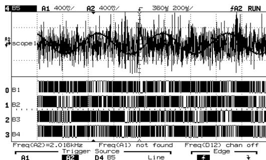
**Figure 6. Acquisition screenshot, one sees DR restriction of the input. Only the digital channels are used in the acquisition algorithm.**
