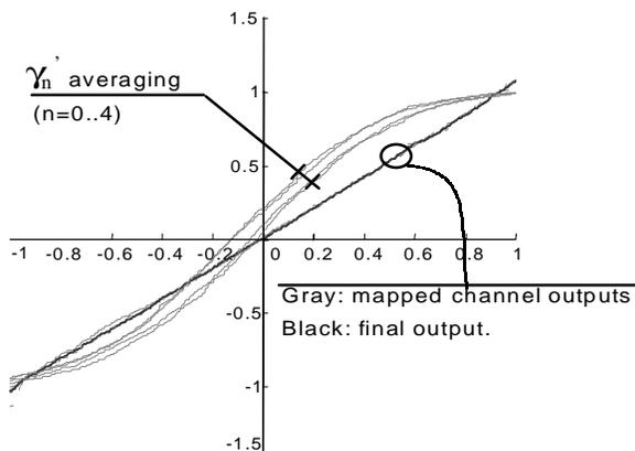
**Figure 7. Outputs from averaging in each comparator and after non-linear statistics mapping.**
