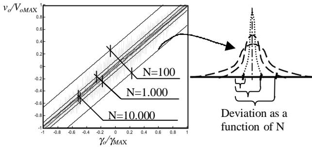
**Figure 3. As averaging depth  $N$  increases, error scattering diminishes allowing higher resolution estimates.**
