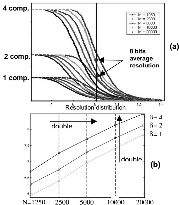
**Figure 8. Parallelism and resolution. Equation 6 predicts min. resolution for a given pair ( $N, \beta$ )**
