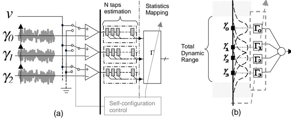
**Figure 5: Acquisition architecture relies heavily on digital processing and self configuration using highly variable analog elements (a). Statistics estimation uses multiple noise references with overlapping regions of influence (b). This way analog offset variation expands the dynamic range (DR).**
