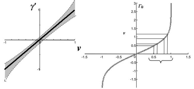
**Figure 4. Non linear noise reference distribution (Gaussian) influence on resolution convergence. For a fixed value of  $N$ , resolution decreases as the DR fringes.**
