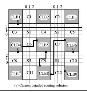
Target two-pin connection:  $A = (CLB1, pin0) \Rightarrow (CLB9, pin1)$   $B = (CLB4, pin0) \Rightarrow (CLB6, pin0)$ Global route alternatives: AG1 = (CLB1 pin0, C3, S1, C4, S2, C7, S4, C12, CLB9 pin1) AG2 = (CLB1 pin0, C3, S1, C6, S3, C9, S4, C12, CLB9 pin1)BG1 = (CLB4 pin0, C8, S3, C9, S4, C10, CLB6 pin0)
