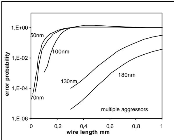
Figure 8. Probability of crosstalk faults as a function of wirelength for different CMOS generations. Multiple aggressor arrangement.
