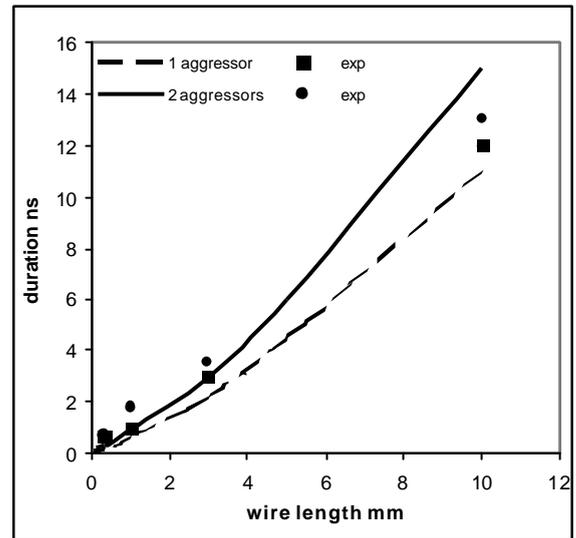
Fig. 3 Duration of crosstalk peak for a 0.25 $\mu\text{m}$  technology Experimental results on a 0.25 $\mu\text{m}$  testchip and simulation
