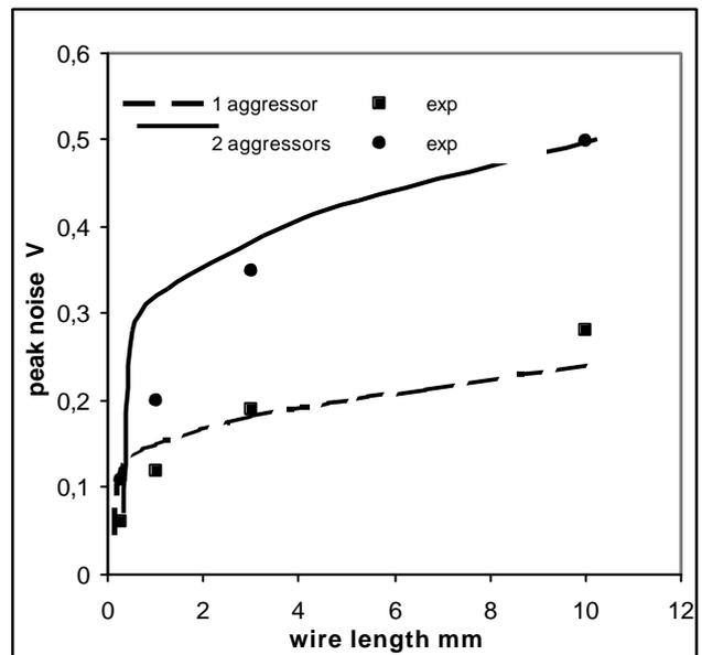
Figure 1. Crosstalk noise as a function of wire length. Experimental results on a 0.25 $\mu\text{m}$  testchip and simulation
