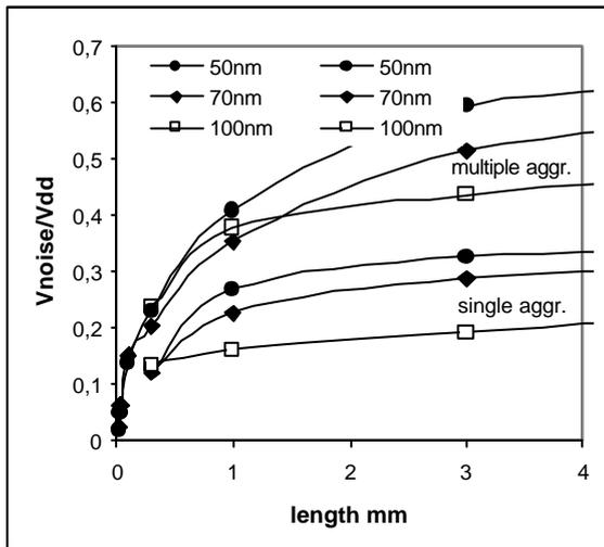
Figure 5. Crosstalk noise peak relative to Vdd for different CMOS generations and for two aggressor arrangements
