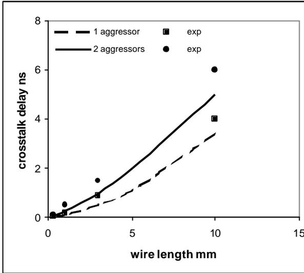
Figure 2. Crosstalk induced delay as a function of wire length. Experimental results on a 0.25 $\mu\text{m}$  testchip and simulation
