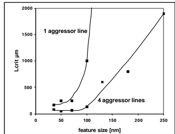
Figure 9. Critical wire length for CMOS technology generations of different feature size
