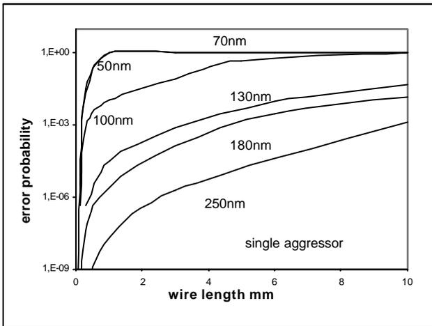
Figure 7: Probability of crosstalk faults as a function of wirelength for different CMOS generations. Single aggressor arrangement
