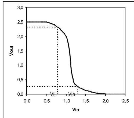
Figure 6. Definition of noise margins for a three input NAND gate from quarter micron technology
