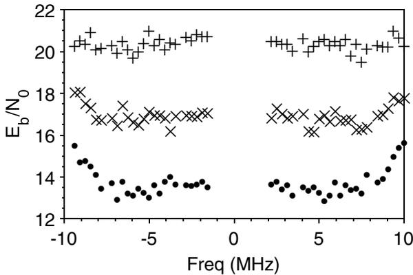
**Figure 4: Energy per Bit to Noise Density Ratio ( $E_b/N_0$ ) of the stochastic (nonlinear) distortion as function of the frequency offset for different levels of the crest factor. From upper to lower curves: crest factors 2, 4 and 5.**
