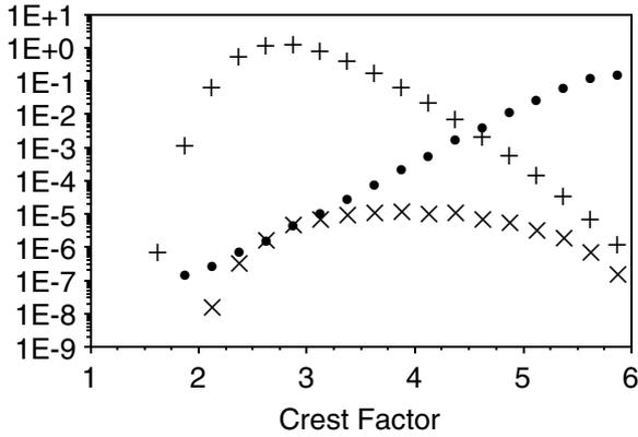
**Figure 1: Analysis for an OFDM signal as function of the crest factor (IEEE 802.11 standard using 64-QAM modulation): ‘+’: probability density function; ‘●’: BER; ‘×’: Product of the pdf and the BER.**
