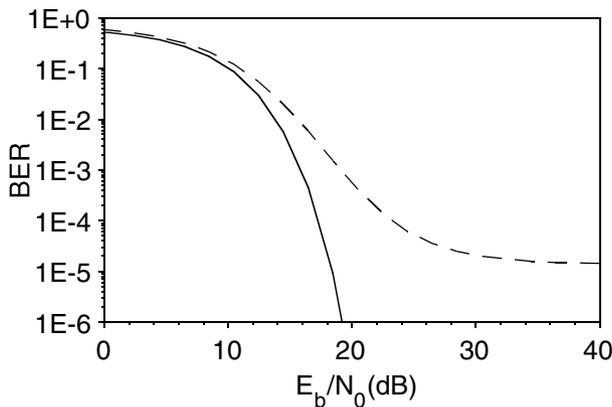
**Figure 6: BER of the IEEE WLAN system as function of the additive noise (expressed in  $E_b/N_0$ ). Solid line: no nonlinear distortion; dashed line: nonlinear distortion included.**
