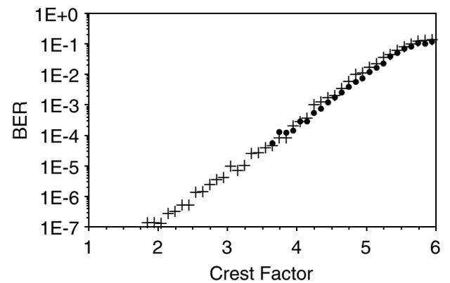
**Figure 5: Verification of the estimated BER as function of the crest factor: '+' : quasi-analytical method (100 experiments/point); '●': Monte-Carlo simulation (5000 experiments/point).**
