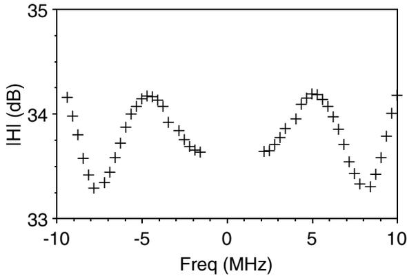
**Figure 3: Mean value of the best linear approximation of the frequency response. The horizontal axis is the frequency offset of a carrier with respect to the 5.25 GHz center frequency. The gap around the carrier frequency comes from the zero carriers as defined by the IEEE standard 802.11.**
