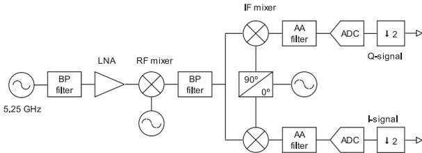
**Figure 2: A 5 GHz WLAN receiver architecture.**
