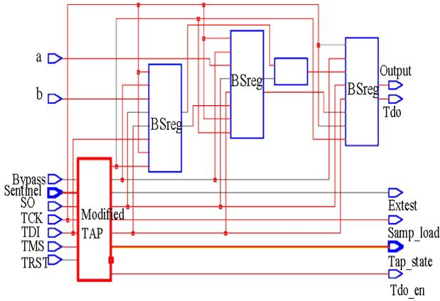
**Figure 5: High level block diagram of modified boundary scan design.**
