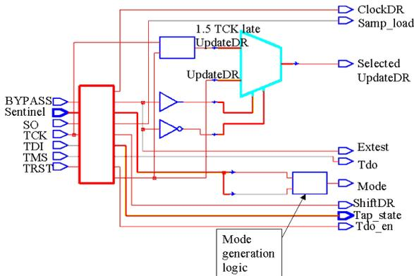
**Figure 6: Detailed description of TAP controller modified for delay testing.**
