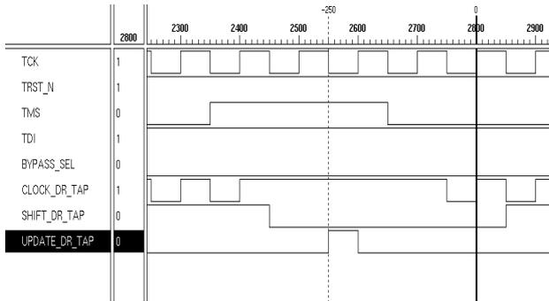
**Figure 2: Timing diagram revealing 2.5 TCKs problem.**
