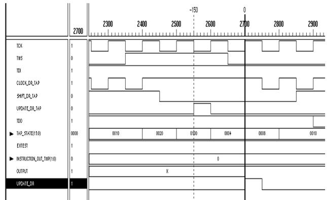
**Figure 8: 1 TCK cycle from UpdateDR to CapturedDR in Asynchronous mode.**
