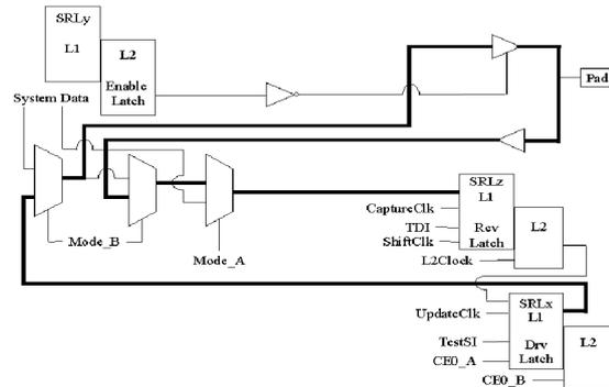
**Figure 1: Testing delay defects on I/O pads using boundary scan.**
