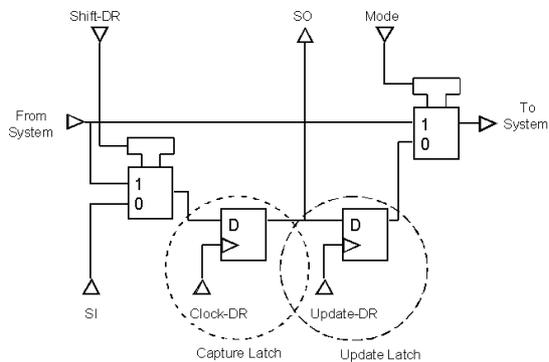
**Figure 3: Detection of delay defects by changing either Capture or Update Latch.**
