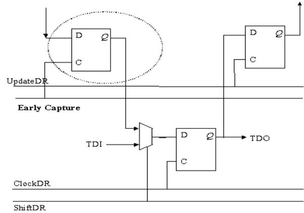
**Figure 4: Delay detection by Early Capture Latch.**
