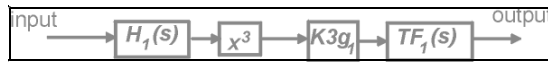
Fig. 2: path from the input to the output of a weakly nonlinear circuit corresponding to the contribution of a one-dimensional third-order coefficient K3g_1 to the overall third-order nonlinear behavior.
