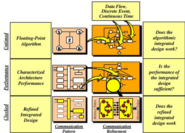
Figure 4. Levels of abstraction for IP integration
