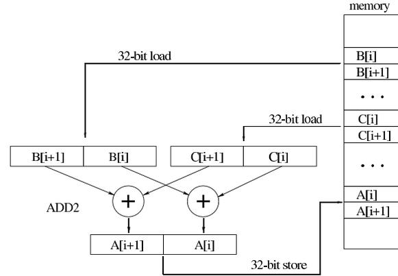
Figure 3. Parallelization of vector addition with SIMD instructions
