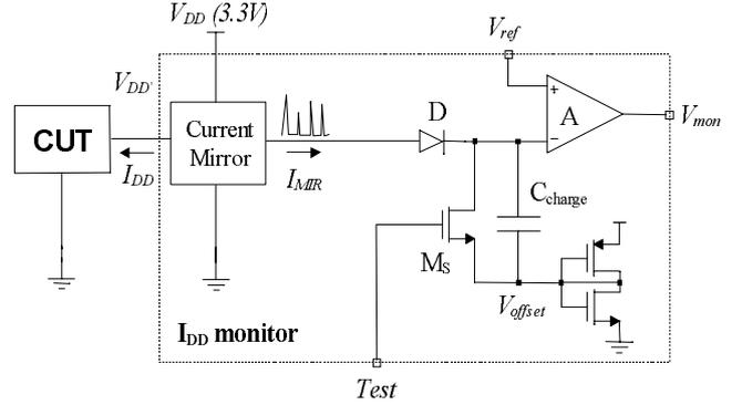
**Figure 2** The proposed transient current monitor
