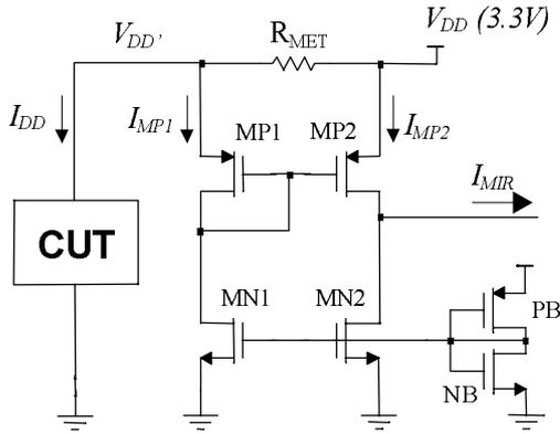
**Figure 1** Current mirror principle of  $I_{DD}$  monitoring
