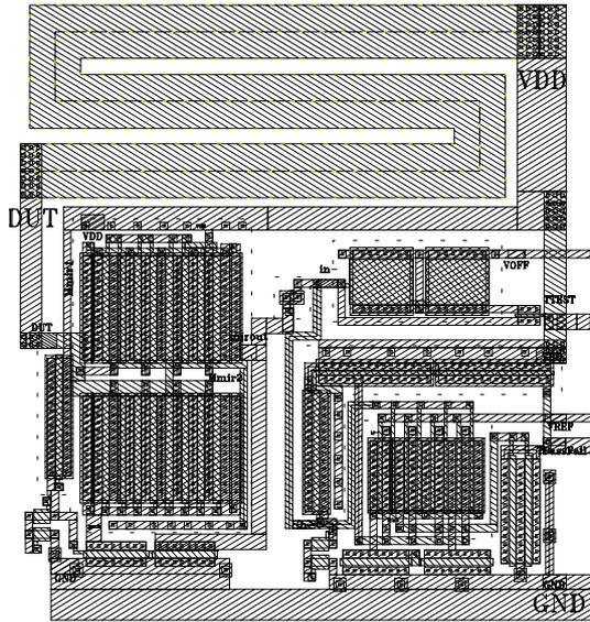
**Figure 5** The core of the transient BIC monitor layout
