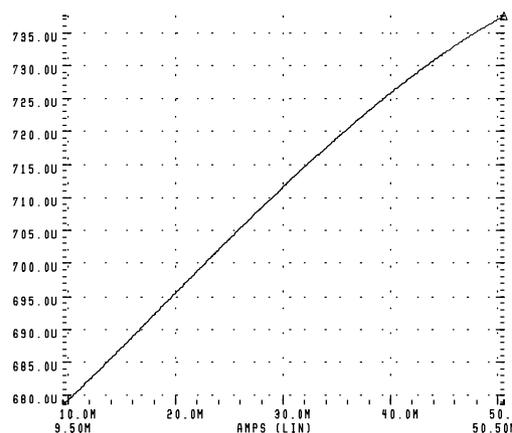
**Figure 4** Linearity of the current mirror for  $R_{MET}$  of  $1\Omega$  and  $I_{DD}$  range from 10mA to 50mA
