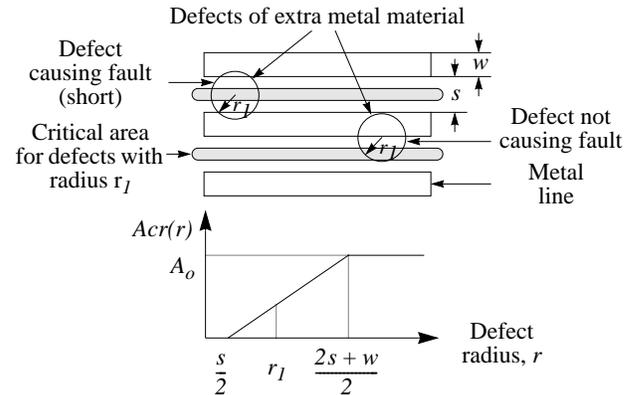
Fig. 2. Critical area function for array of metal lines.
