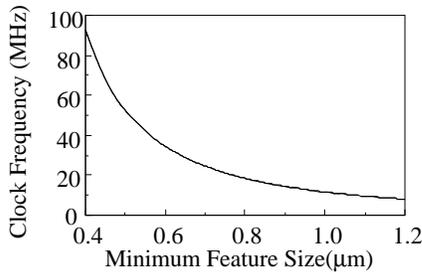
Fig 7. Clock frequency vs. minimum feature size.
