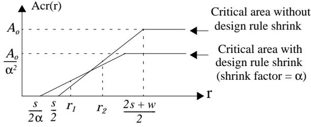
**Fig 3.** Critical area vs. defect radius for original and shrunk array of metal lines.
