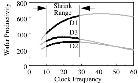
Fig 8. Parametric plot of wafer productivity vs. clock frequency as design rule shrink increases.
