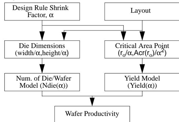
Fig 1. Analysis flow of shrink on wafer productivity.
