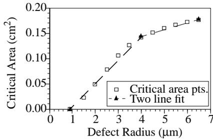
**Fig 4.** Two linear function fit of critical area curve.
