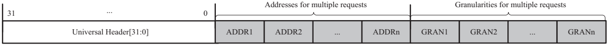
Fig. 3: The new request packet header layout of SPMR with multiple memory requests, each request needs a separate ADDR and GRAN field.
