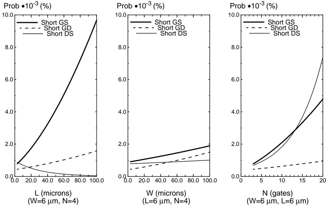
Fig. 4: Predicted probabilities of shorts for interdigit transistors
