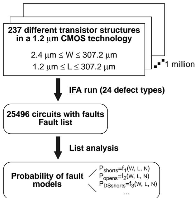
Fig. 1: Model derivation flow
