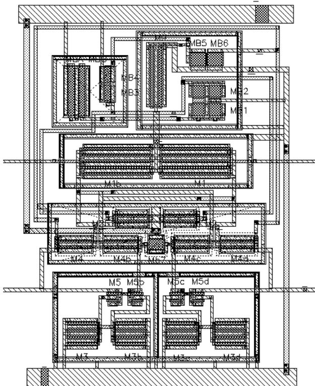
**Fig. 6: Layout of the fully-differential opamp**
