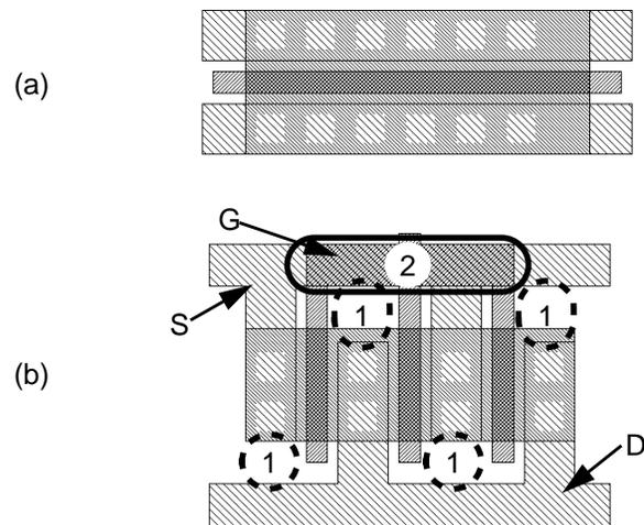
Fig. 2: Different transistor shapes: (a) rectangular, (b) interdigit.
