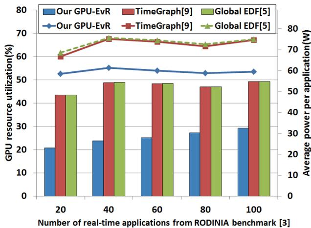
Fig. 5: GPU resource utilization and average power per application in 28nm technology
