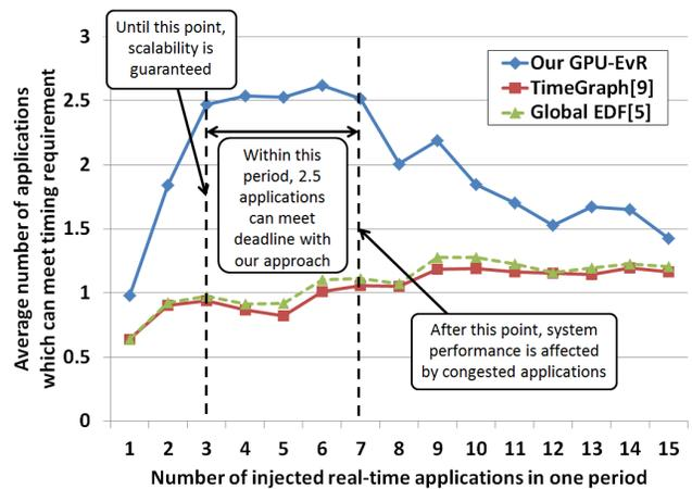
Fig. 6: Scalability comparison of GPU-EvR compared to [5], [9]
