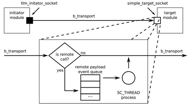
Fig. 1. Local and remote TLM transaction flow
