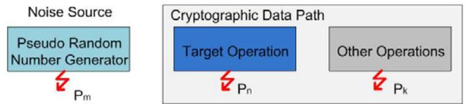
Figure 4: : Increasing resistance to attacks by adding high noise level
