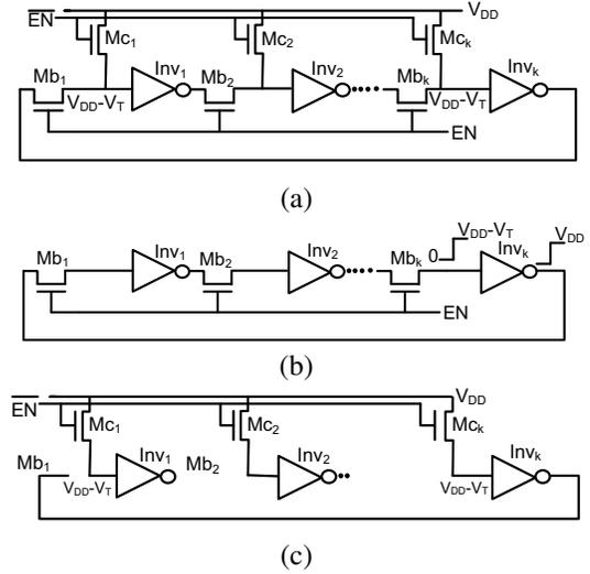
Figure 3: (a) Aging-Resistant RO (ARO), (b) Oscillatory mode, and (c) Non-oscillatory mode.
