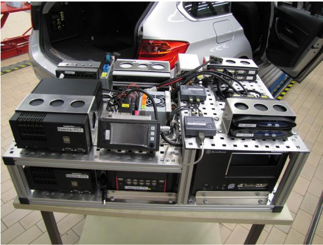
Fig. 1. Hardware Setup Mounted on the Rack
