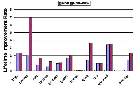
Fig. 5. The lifetime improvement rate of the multiple dirty bit (MDB) and read before write (RBW) schemes.
