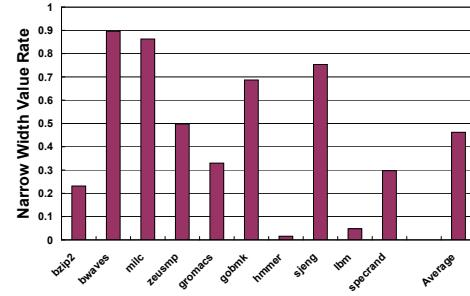
Fig. 3. The percentage of the narrow-width values (leading zeros) in the last level cache.
