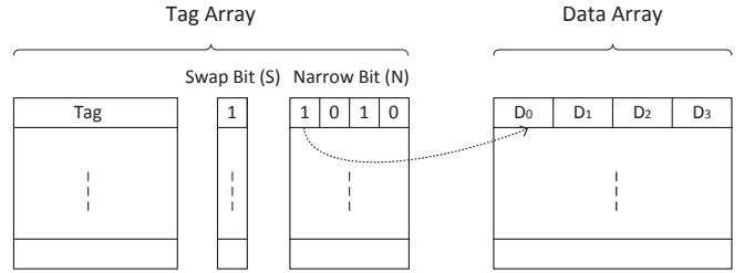
Fig. 2. Block diagram of the proposed non-volatile cache design.
