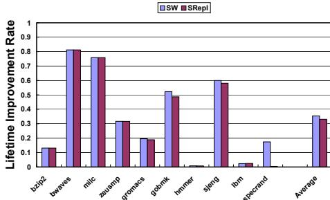
Fig. 4. The lifetime improvement rate by applying the swap on write (SW) and swap on replacement (SRepl) schemes.
