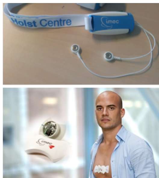
Fig. 1. Single-lead ECG necklace and ECG patch for determining energy expenditure.
