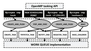
Fig. 5. Design of tasking support
