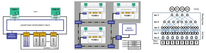
Fig. 1. On-chip shared memory cluster template Fig. 2. Multi-cluster architecture and global address space
