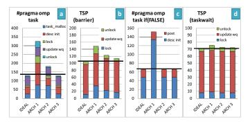
Fig. 7. Breakdown of the time spent in high-level OpenMP services
