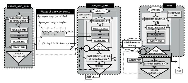
Fig. 4. Design of task scheduling loop
