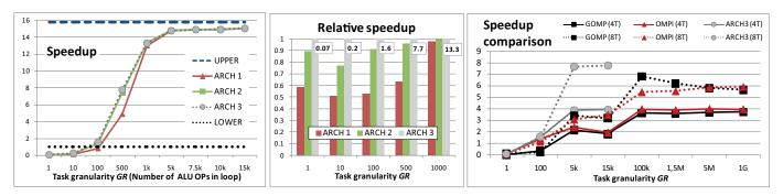
Fig. 8. Parallelization speedup for increasing task granularity (a,b) and against existing OpenMP runtimes (c)
