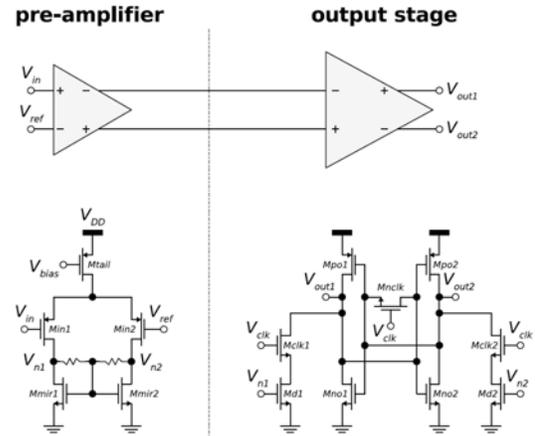
Fig. 6. Schematic of the clocked comparator example circuit used to illustrate the stochastic reliability analysis.
