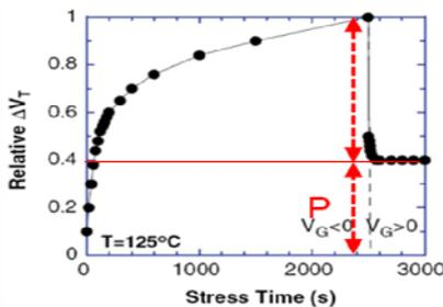
Fig. 2. BTI degradation showing partial recovery when the stress is removed, still leaving a permanent degradation  $P$ .
