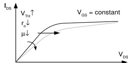
Fig. 1. Time-dependent variation of the characteristics of a transistor due to Hot-Carrier and BTI degradation [2].
