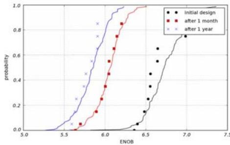
Fig. 14. Normal probability plot of the ENOB of the flash ADC for 100 random samples evaluated with an hierarchical simulator (solid lines) and 10 samples evaluated with full system simulations (markers) for the fresh circuit and the aged circuit after 1 month and 1 year.
