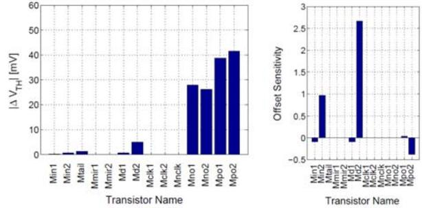
Fig. 9. Analysis of the aging-induced  $V_T$  shift of every transistor in the comparator (left), and sensitivity of the offset to the  $V_T$  shift of every transistor (right). Both aspects are needed to get a clear view on the impact of aging on circuit performance.
