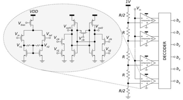
Fig. 12. Flash analog-to-digital converter in which the clocked comparator is used to compare the input signal with the reference values.
