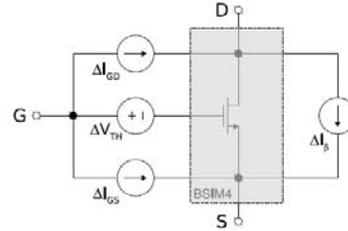
Fig. 5. Equivalent subcircuit for a degraded transistor with the original transistor being modeled by standard models such as BSIM4 and the time-dependent aging degradation being modeled by the additional dependent sources around the transistor. Such subcircuit model can be used in standard SPICE simulators.
