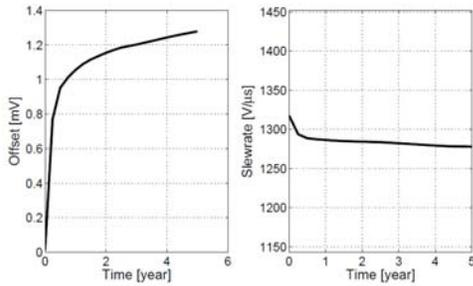
Fig. 8. Aging-induced circuit performance shift in the comparator: the input offset is very sensitive to circuit aging, while the slew rate remains more or less constant.
