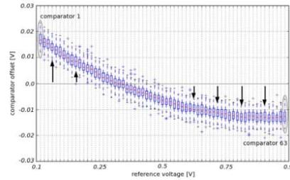
Fig. 13. The input-referred offset voltage for each flash ADC comparator after 1 year of stress and for 100 random samples, all evaluated with the comparator subblock model. The arrows indicate the offset shift between the initial state and after wear-out.
