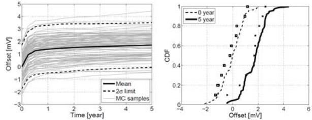
Fig. 9. Comparator offset as a function of the stress time for 100 random samples evaluated with the DOE-based stochastic reliability analysis (left). Cumulative distribution function of the offset for a fresh circuit (time  $t=0s$ ) and for an aged circuit (time  $t=5years$ ), showing both the results of 100 samples of the the DOE-based stochastic simulator (lines) versus 10 random samples with the MC-based simulator (markers) (right).
