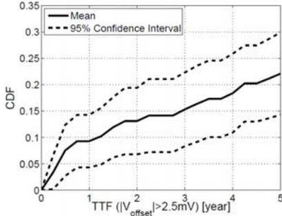
Fig. 11. The cumulative density function for the time to failure of the comparator circuit (together with 95% confidence interval bounds). A circuit is considered to fail if the offset surpasses 2.5 mV.
