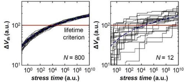
Fig. 3. Due to the discrete nature of the trapping and detrapping events, the time-dependent BTI-induced  $V_T$  shift becomes stochastic for small devices in sub-45nm CMOS [17,18], hence also making the lifetime being spread stochastically.
