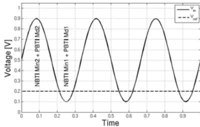
Fig. 7. Stress waveform applied to the example comparator circuit. The regions of degradation for the different transistors are indicated.
