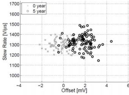
Fig. 10. The stochastic performance space for the offset and the slew rate for a fresh circuit and a circuit after a stress time of five years for the comparator example circuit in 32nm CMOS.
