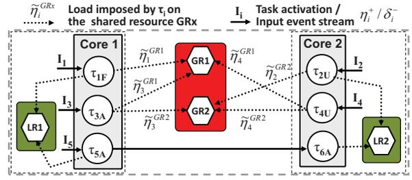
Fig. 1. Multi-mode multi-core system during a transition phase.
