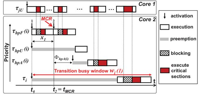
Fig. 3. Scheduling example for a task  $\tau_i$  during a mode change where *MCR* coincides with the 2nd activation of the higher priority finished task.
