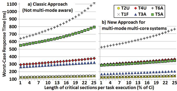
Fig. 4. Tasks' WCRTs depending on the critical sections length: a) current design practice; b) our approach for multi-mode multi-core systems.
