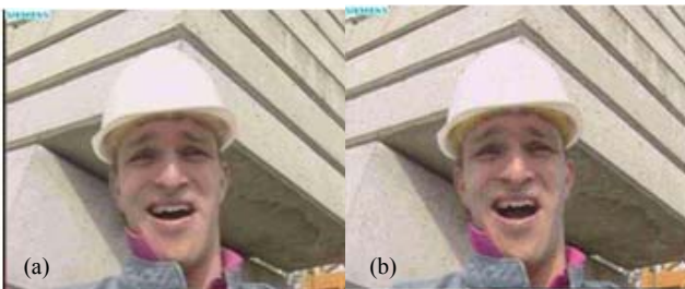
Figure 7. Barely acceptable sequence quality for (a) bank protection after filtering (b) HOB protection. The filter artifact may be observed at the edges for bank protection. Snowy background may be observed in HOB protection due to lower bit corruptions.
