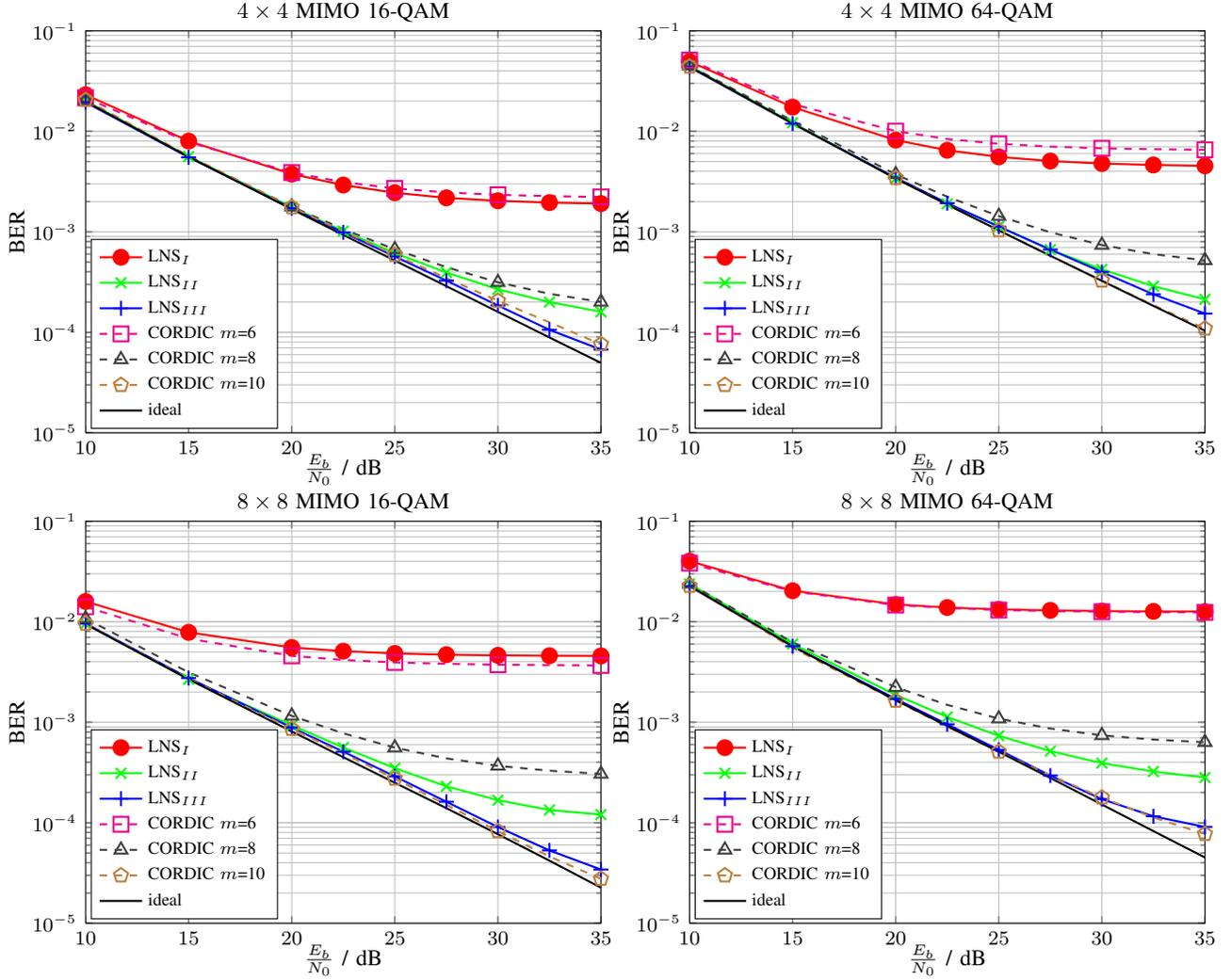
Fig. 6. Uncodes BER performance at the receivers side of the three different LNS-based QRD realizations. The CORDIC is simulated in floating-point, where  $m$  denotes the number of micro-rotations.
