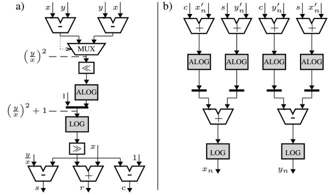
Fig. 4. Data path of LNS-based QRD with a) GR1 and b) GR2 and  $x > y$ . The solid, dotted and dashed lines depict the data flow, the control signal and interim results, respectively.  $x'_n$  and  $y'_n$  denote the unrotated inputs as well as  $x_n$  and  $y_n$  are the resulting outputs.
