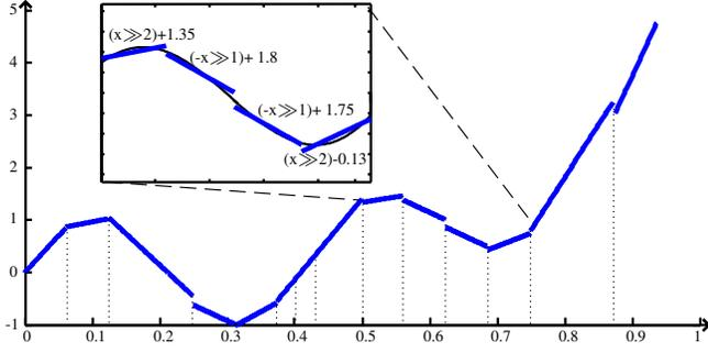
Fig. 3. Example of nonuniform multiplier-less piecewise function approximation.
