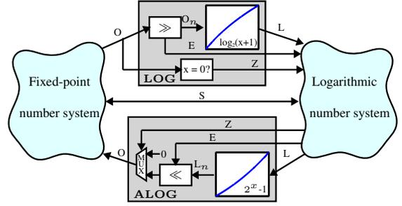
Fig. 2. Architecture of LOG and ALOG converter for number system transformation.
