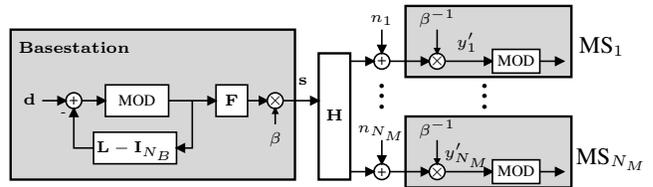
Fig. 5. THP structure in the base station for downlink transmission with decentralized mobile stations (MS).
