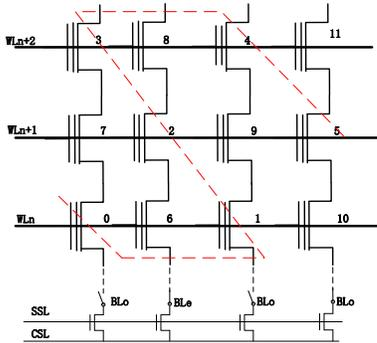
Figure 9. Testing sequence for checkboard pattern.
