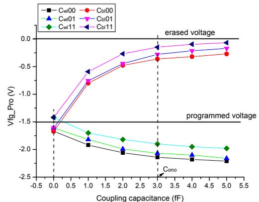
Figure 5.  $V_{th\_shift}$  induced by the coupling capacitors.
