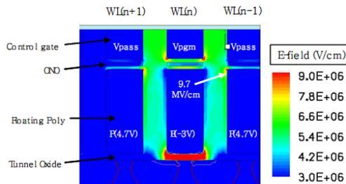
Figure 2. The simulated electric potentials of three neighboring cells with the cell WL(n) applied a programmed voltage and two neighboring cells applied a pass voltage.[8]
