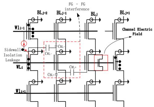
Figure 4. SPICE model and functional behavior of the interference defects.
