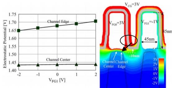
Figure 3. Simulation results depicting the potential distribution of the channel of a selected cell at the center and the edge due to the voltage of the FG of its neighboring bit-line cell.[9]
