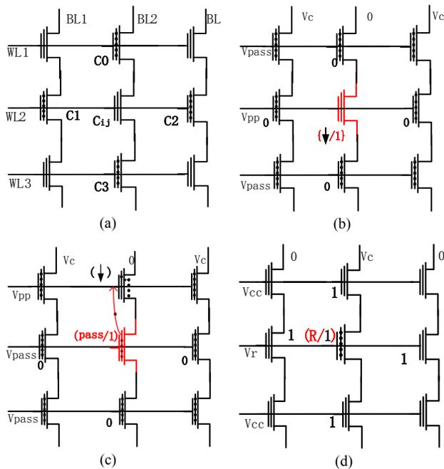
Figure 8. (a) a typical 3x3 NAND Flash array; (b) the test condition for the PRIF fault; (c) the test condition for the SFIF fault; and (d) the test condition for CFIF fault.
