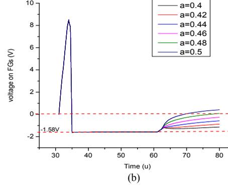
Figure 6. (a) The voltage applied on the CGs; (b) the simulated voltage on the FG of the victim cell.
