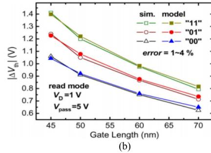
Figure 1. (a) The cross-section of an EEPROM cell with two adjacent cells; (b) The  $V_{th}$  shift of the programmed cell ( $V_{th} = 2$  V) versus the gate length of the memory.[7]
