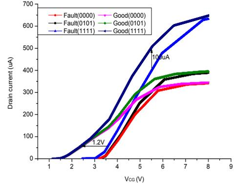
Figure 7. The simulated current flowing through the victim cell w.r.t. its CG for the faulty case and the good case respectively for different aggressor background patterns.
