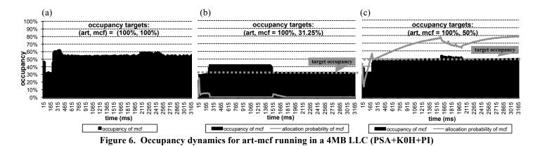
When a PI controller is incorporated with PSA+K0H, the overflow and underflow are monitored dynamically and the allocation probabilities are adjusted to achieve an accurate occupancy within 1%. The 0% requested occupancy however results in a 6% overflow, because of the underlying limitation that we don't have a mechanism to bypass the cache and some lines do remain in cache though they are marked LRU.
