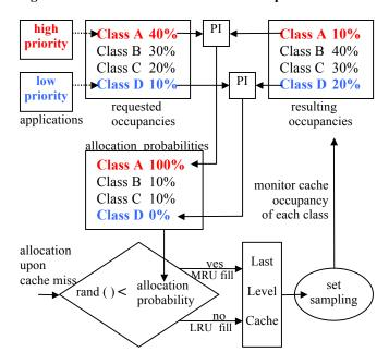
Figure 3. PCASA Architecture incorporating PI controllers
