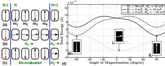
Fig. 1. (a) AF-line moves information; (b) an AF-line has a new input, and an external clocking field is used to facilitate re-evaluation of the line; (c) as the field is removed, devices relax along their easy axes; (d) Energy landscape of a representative magnet when subjected to different field combinations.
